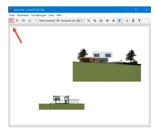
The prepared PDFs can be loaded and organized in Lexo 2D. The saved Lexo 2D file always shows the current state of the integrated PDFs when it is opened. Changes made in Lexocad can therefore be quickly transferred to the PDF.
