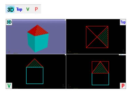
**3D:** The model is displayed as an axonometry. It is however possible to define different views:
