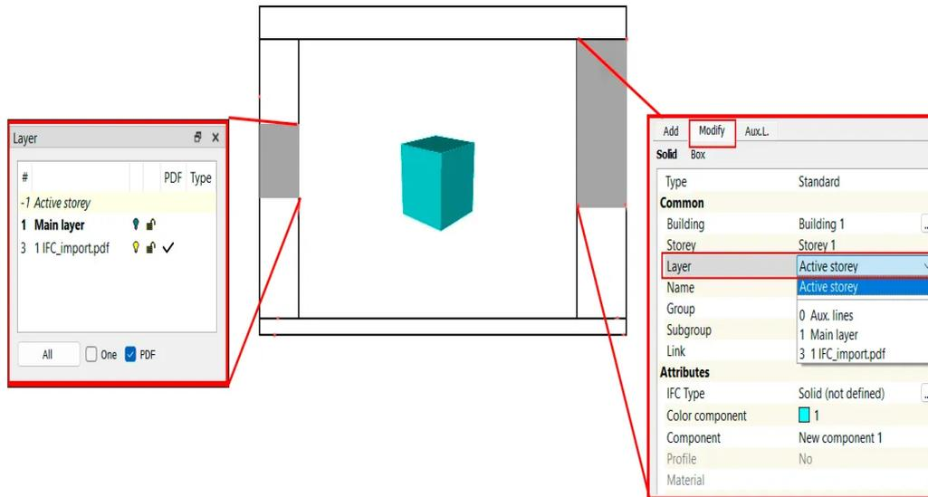
A double-click on a layer activates it and displays it in bold type. In the Modify area (right menu), it is possible to modify the layer of an active element.
