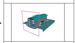
The cutting plane can be moved with " **Shift** + Arrow".
