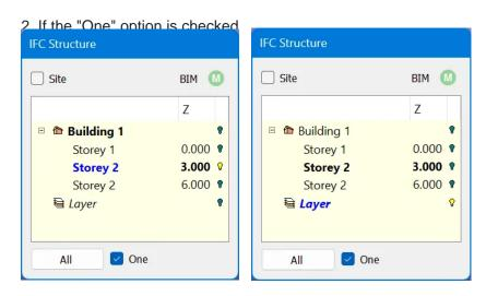
In this case it is possible to display only one floor at a time, all others will be hidden If floor 1 is displayed and the light bulb of floor 2 is clicked on to display it, floor 1 will be hidden
